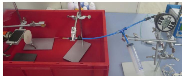
Figure 1: Set-up of measurement equipment for impact force and system pressure
