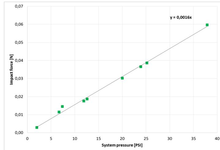
Figure 2: Correlation of maximum impact force and system pressure during manual actuation at different effort
