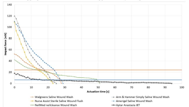
Figure 4: Impact force changes during emptying of available wound wash products
